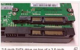
2.5-inch SATA drive on top of a 3.5-inch SATA drive, close-up of data and power connectors
