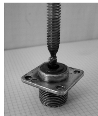
Fig. 3 – Detail of the threaded rod and SO-239 fitting.
