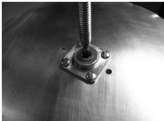
Fig. 4 – Threaded rod/SO-239 bolted in place.
