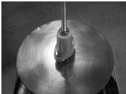
Fig. 4 – Ceramic insulator to stabilize soldered joint.
