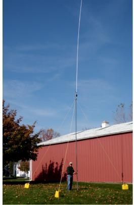
Ed Frac (AA9WW) tried out the new Comet vertical antenna he assembled for portable use. It requires no radials – but then neither do rain gutters.
