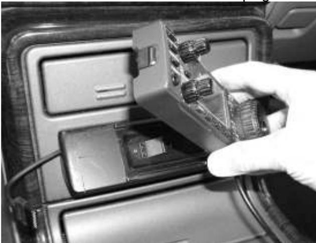
A little sanding, flat black paint and mounting of the control head bracket completed the “insert mount”.
