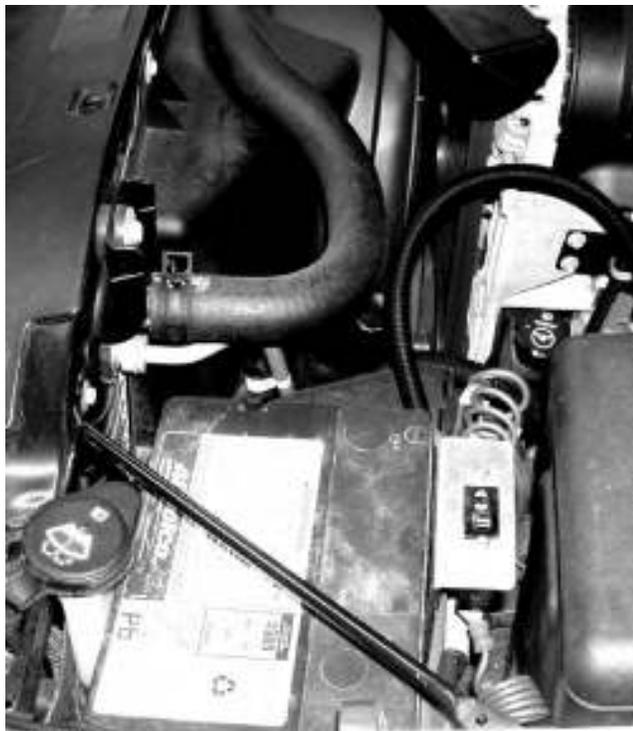
**Here the circuit breaker assembly is installed with the positive lead connected to the battery positive terminal. A GM dealer or parts house can provide "long" battery bolts to accommodate the addition of the lugs. Note the battery accessory power box in the upper right of the photo.**
