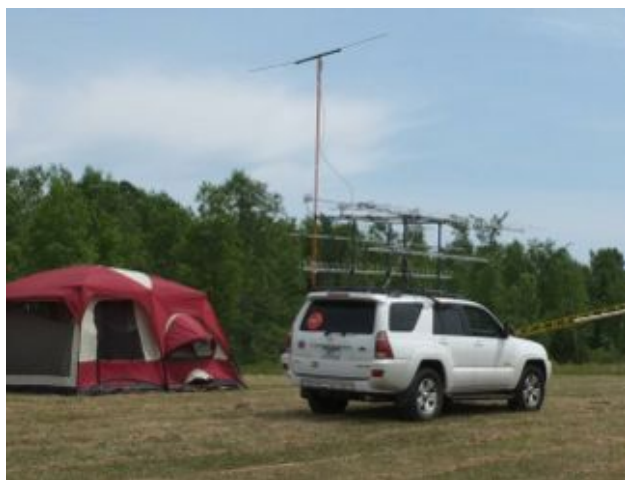
The W9FZ "Rover" at the ORC Field Day 2012. The antennas mounted on the roof rack are for 50 MHz (6 meters), 144 MHz (2 meters), 220 MHz, 440 MHz, 900 MHz, and 1.2 GHz bands.
