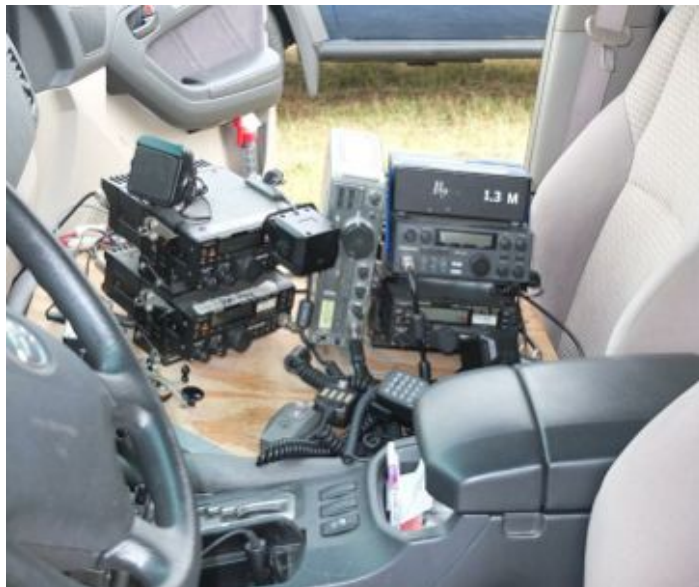
Inside the W9FZ "rover". Rigs and transverters permit operation on multiple VHF+ bands.
