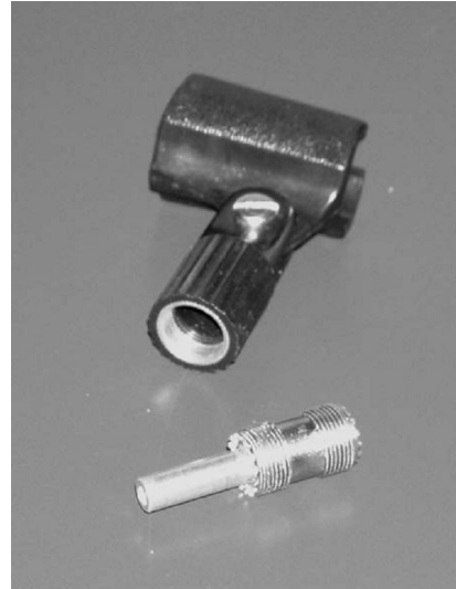
The mic holder was available from Tower Electronics for about a dollar and the 24 t/in thread fits a coax coupling.
