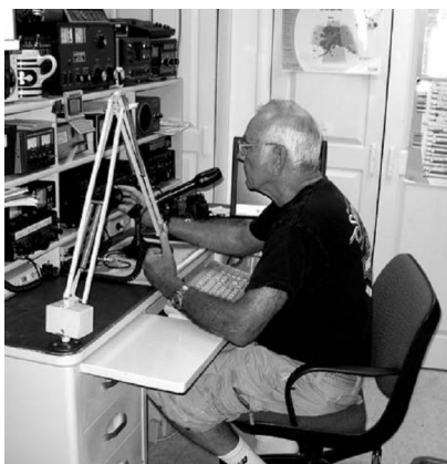
A 1/2" pipe nipple and floor flange is used to assemble a secure desk swivel mount for the "mic econo-arm"
