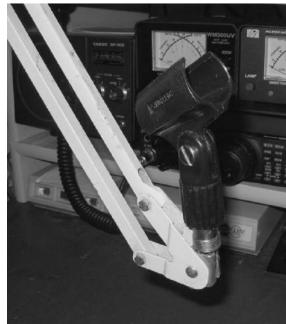
The adapted mic holder is shown secured in the extension arm clamp.
