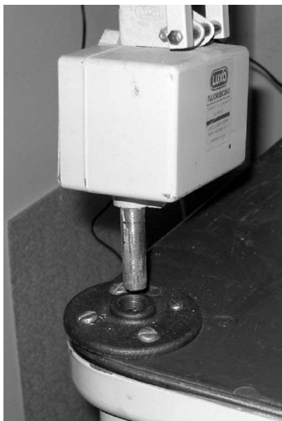
A 1/2" pipe nipple and floor flange is used to assemble a secure desk swivel mount for the "mic econo-arm"
