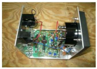
The WM-2 has three power ranges of 100mW, 1W, or 10W with a claimed accuracy of 5% of full scale. It is powered from either an internal 9V battery or an external power supply. The meter measures both forward and reflected power so you can use the readings that you make to calculate SWR if you wish.
