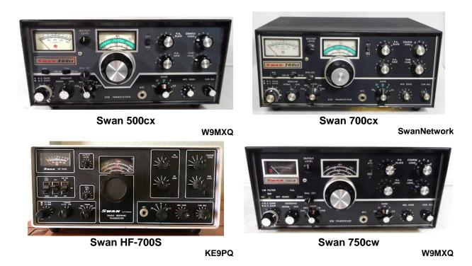
The HF-700S is more toward a Cubic Communications product (Swan's parent company) in panel design and cabinetry. And, unlike the other three, only the 700cx used the 8950 final tubes – as noted, above.
