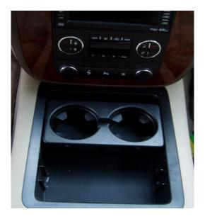
There was however a compartment with a movable drink holder. The drink holder could be inserted into either a forward or rear position within the compartment.
