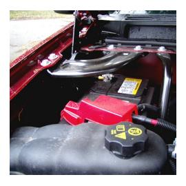
Finally I noted an opening in the firewall at the rear of the right fender under the hood along the side of the battery. It worked out perfectly to route the #10 stranded wire from the battery to the units under the rear seats.
