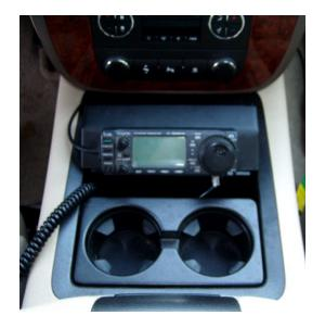
This allowed for the control head to be conveniently mounted for viewing and operation while not interfering with the drinks.
