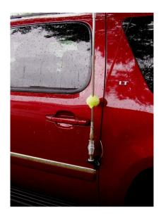
Temporally the HF antenna was mounted to a rear side door using a "lip mount". While this arrangement works OK and allowed me to check into the FL-Milwaukee net on 14.290 it just does not seem very secure and I will be replacing the mount with a type of hitch mount.
