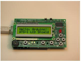
Arduino LCD terminal shield developed by Gary Sutcliffe (ATS1W9XT)
