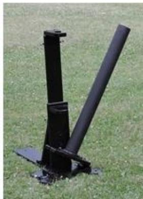
I've seen some solutions where a length of pipe is attached to a board and placed under a vehicle tire. This solves the anchoring problem but doesn't help with the tilting problem. Searching around I found a very nice solution that was built by KL7JR, "The One Person Antenna Raiser" (<http://www.hamuniverse.com/kl7jrantennaraiser.htm>). This was along the lines of how I was thinking of solving the problem.
