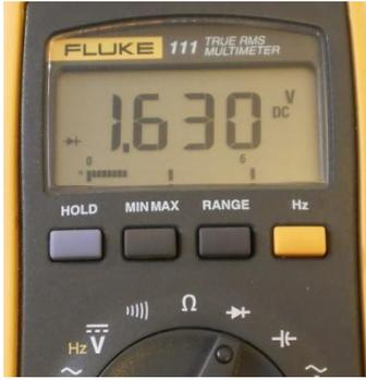
Can't remember if it is the long or short lead on an LED which is the cathode? Why not check it with the DMM? Just connect the test leads across the LED and see if it lights up. If not, reverse the leads and take note to the negative lead and the length of the LED lead it is connected to. (It will not be full brightness and therefore you must be sure you are looking at it straight on and not off to the side as in the picture.)
