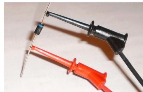
still holds true using a DMM except for one thing. In many cases, the DMM, because of the processor it uses, doesn't provide enough voltage to forward bias a diode while in Ohms. That is why there is a separate "Diode
