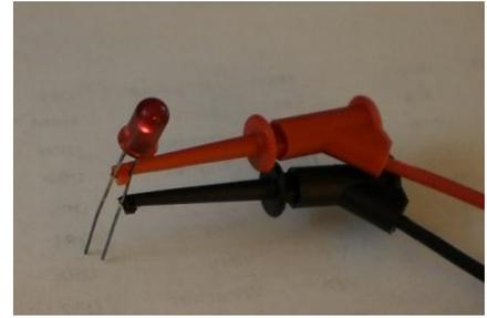
Again, the DMM will display the voltage it takes to forward bias and turn the LED on. In this case it is 1.63 volts which is enough to turn it on but not to full brightness which is usually around 2.2 volts.
