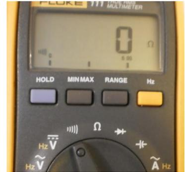
Check" you can do just that. You connect your test leads across the contacts you want to check; activate the relay, and LISTEN for a steady tone. When you release the relay, the tone should disappear. You may check this function of the DMM just by touching the probes together, or if you're
