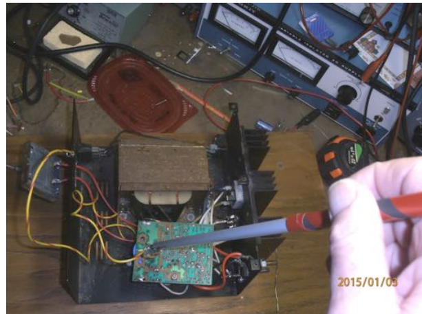
To use, simply attach the alligator clip to chassis and touch the connected end probe to the filter capacitor +..
