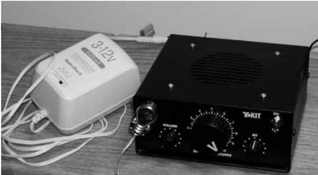
**The TenTec 1340 is a single bander transceiver priced at about \$100 and produces 4 watts using a wall wart power supply**
