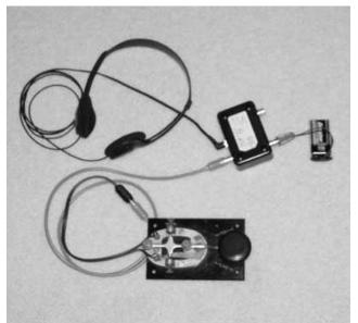
The Pixie 2 is shown here with a WWII J38 key, headset and 9 volt battery – only the antenna and operator are missing
