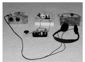
N9JIY's home-brew CW RCVR on the left and transmitter on the right. The unit in the middle is a manual DPDT transmit-receive switch. Minimal investment of dollars and maximum output of thrilling contacts with only 1 watt.
