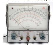
sistant circuit, you will conclude it will have a negligible effect, and therefore provide an accurate measurement. A value of 10 meg ohms for input impedance is now the accepted standard.
