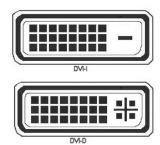
cable into it and you are home free, though you will be using an old, analog monitor. If they do not, the connectors will usually be one of the two digital types shown here. If you have a DVI-I connector on the back of your computer, you can purchase a little adapter that will plug into it and accept a VGA
