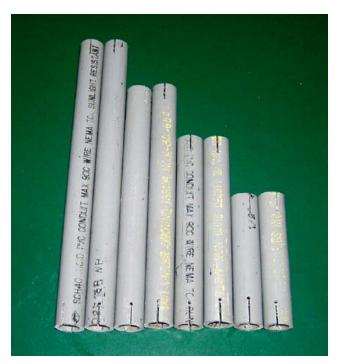
The conduit was cut into 4", 6", 8" and 10" lengths with the shorter spacers to be used nearest the center balun.
