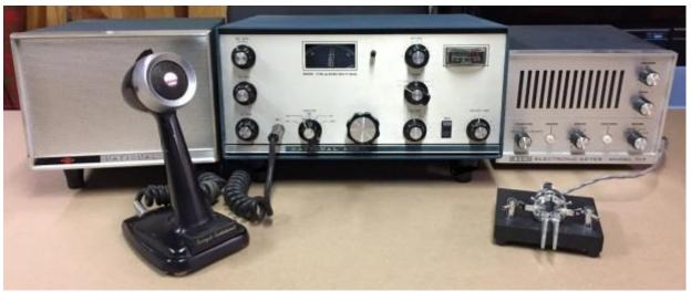
Left to Right are the National NCX-A AC Power Supply/Speaker, the National 200 HF Transceiver, and an Eico 717 Electronic Keyer that shows well with this station. Also shown are the very popular, at the time, Turner 254C "Crystal SSB Microphone." At the lower right is the much later Bencher BY-1 Keying Mechanism.
