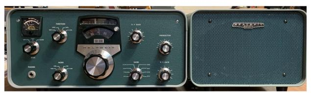
Heathkit SB-300 HF CW-SSB-AM Receiver<sup>1</sup> Shown with Heathkit SB-600 Speaker Console
