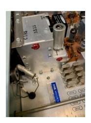
This is a picture from the right front looking at the PTO chassis with its single tube. The red marks on two of the assembly screws indicate assembly at Heathkit for best stability. This was why sophisticated test equipment was not required to align this radio after assembly. Requirements were for a Vacuum Tube Voltmeter, the Calibrator in the SB-300, and another receiver used to align the calibrator.
