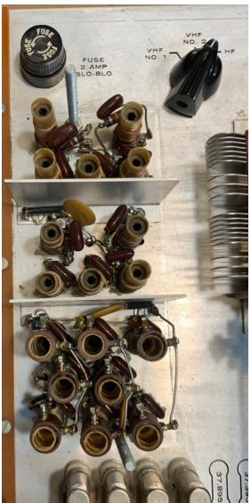
Alignment Coils – With Shield Cover Alignment Coils – Without Shield Cover Alignment Coils Area of the Chassis – See Top View for Location
