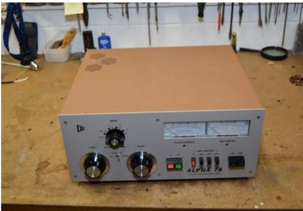
The amp was originally designed to run at a maximum of 1 KW output, to match the FCC requirements in 1980. However, now Alpha provides an input circuit update that allows reaching the current legal limit of 1500 watts output. I installed this mod and tested the amp.
