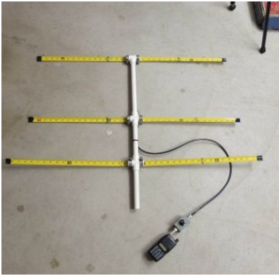
Fox hunting equipment: homebrew handheld yagi antenna and HT with attenuator attached.
