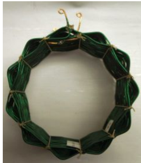
Fig 2. Two different views of L1. On the left, the large amount of air space between the windings can be seen, a desirable characteristic of rook-wound coils that leads to less capacitance between windings and a higher Q. On the right, the coil pattern is evident from the over 1 – under 2 winding. I used nylon thread to tie the windings together before sliding the coil off the winding form. Then I used a narrow band of epoxy on the outside of the coil to anchor the windings permanently.
