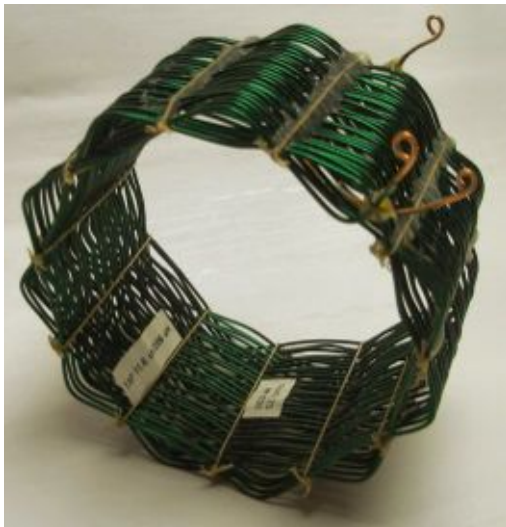
Fig 2. Two different views of L1. On the left, the large amount of air space between the windings can be seen, a desirable characteristic of rook-wound coils that leads to less capacitance between windings and a higher Q. On the right, the coil pattern is evident from the over 1 – under 2 winding. I used nylon thread to tie the windings together before sliding the coil off the winding form. Then I used a narrow band of epoxy on the outside of the coil to anchor the windings permanently.
