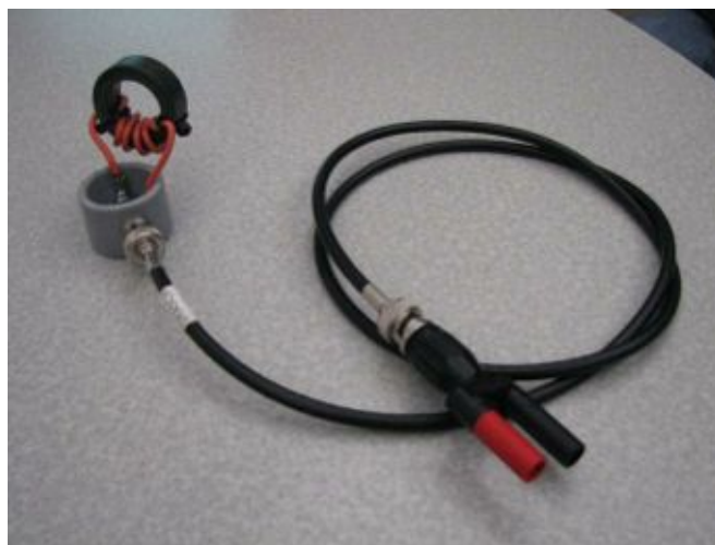
Photo 2: K9DJT's homebrew RF sniffer.
