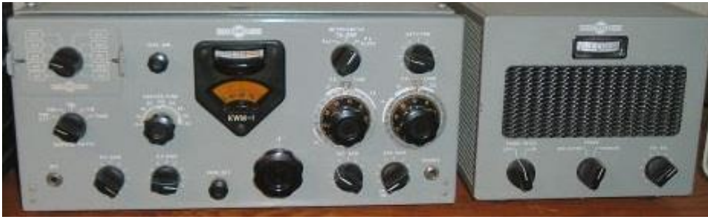
The KWM-1 Transceiver and the 312B-2 Speaker (the 312B-2 included a Speaker, Wattmeter, and Phone Patch)
