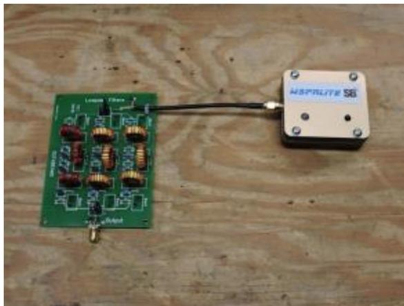
The device is called the WSPRlite (<http://www.sotabeams.co.uk/wsprlite>). It's a 200 mW WSPR transmitter that supports the 20m and 30m bands, and with the added Low Pass Filter kit it can operate on the 40m, 80m, and 160m bands. The WSPRlite transmitter comes assembled in a 2"x2"x0.75" enclosure. The only interfaces are a micro USB port for power and configuration, an SMA connector for an antenna, and a button to start transmitting.
