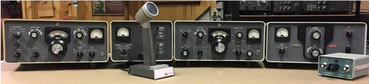
**Collins 32S-3 Transmitter, 312B-4 Console, 75S-3B Receiver, 30L-1 Linear Amplifier
