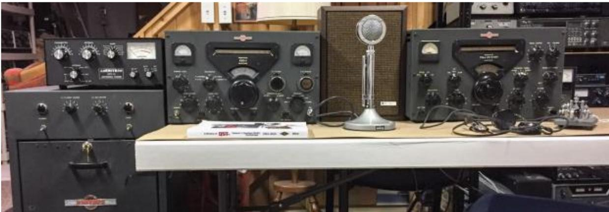
**Left to Right are the KWS-1 Transmitter Power Supply (floor mounted in this installation), the KWS-1 Transmitter RF Unit, the temporary Speaker (more about this below, in the text), and the 75A-4 Receiver. You will also note the Ameritron ATR-15 Antenna Tuner on top of the Power Supply, the Astatic D-104 Microphone, an old set of Lincoln Headphones (“Cans”), and a Vibroplex “Bug” Keying Mechanism.**
