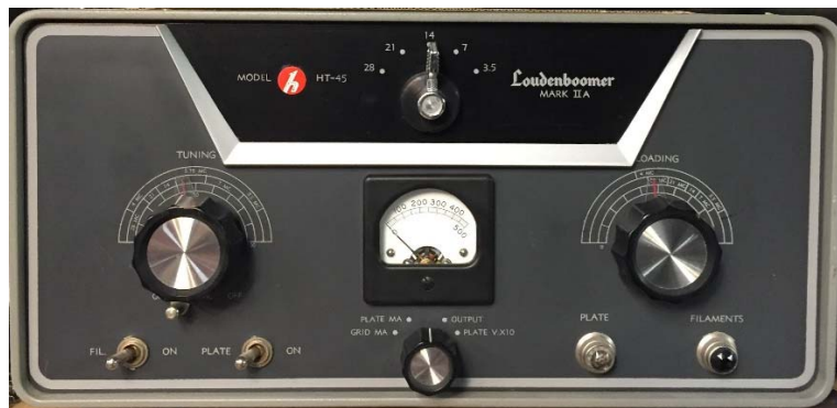
Hallicrafters HT-45 Mark IIA 80-10 Meter Linear Amplifier (Hallicrafters P-45 High Voltage Power Supply is Separate.) (W9MXQ Shack Photo)
