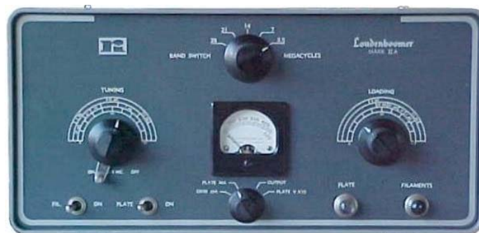
Radio Industries Loudenboomer Mark IIA 80-10 Meter Linear Amplifier (Radio Industries PS-2A High Voltage Power Supply is Separate.) (Radio Industries Loudenboomer Operating Manual)
