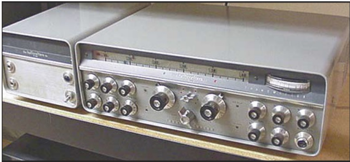
Hallicrafters FPM-200 HF Transceiver with P-200 AC Power Supply HF Coverage of 80-10 Meters
