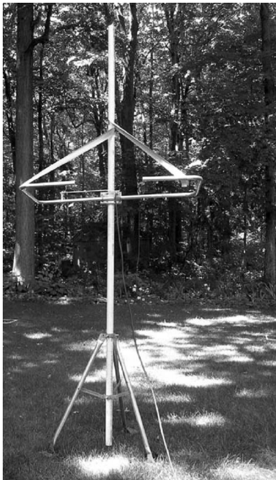
Temporary setup in the back yard for squalo tuning. Duct tape is supporting the squalo in the horizontal position.
