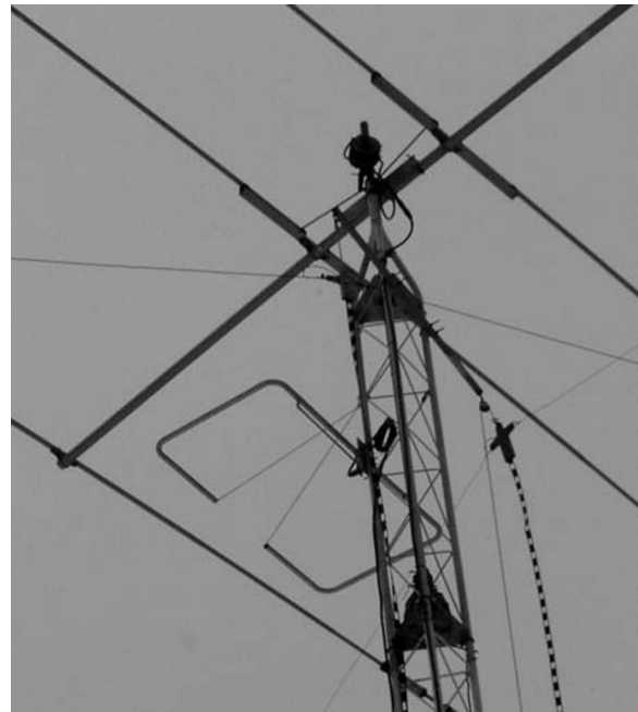
The Lawn Lounge Chair Squalo is shown hard mounted to the tower for horizontal polarization (SSB) with the opening toward the East.
