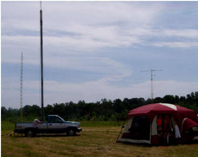
Mark Potash (KC9GST) constructed a special truck mounted motor driven 30' tower for the 6 meter station manned by Gary (N9UUR) and Jeananne (N9VSV) Bargholz.
