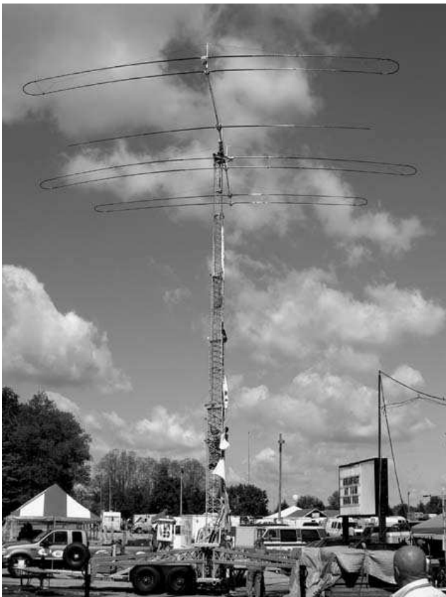
You heard of the Stepper beam antenna. Now you have seen one – big huh?
