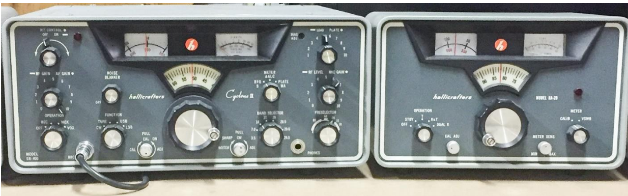
Hallicrafters SR-400 Cyclone II HF Transceiver with HA-20 “DX Adapter” (Remote VFO)
