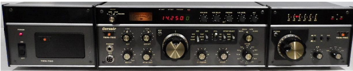
The original version Ten-Tec Corsair HF Transceiver Note Logo above Phone Jack (left) replaced by an added control on the Corsair II.
