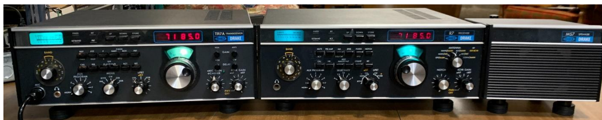
Drake TR7 HF Transceiver (Left) with Drake R7 HF Receiver Shown with SP7 Speaker Console (Right)
