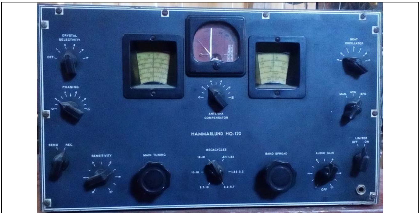
Hammarlund HQ-120X Receiver, manufactured in 1941. The front panel does not have the "X", the model number is marked on the chassis. Crystal filter controls in upper left. Calibrated band-spread dial on right. The front panel is black; the lighting makes it look blue. Photo credit: W9JL
