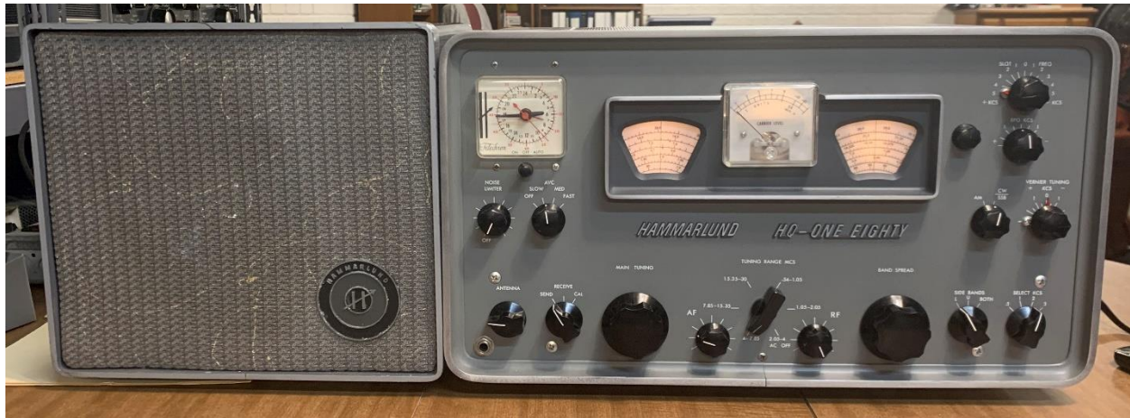
Hammarlund HQ-180 General Coverage Short Wave Receiver (1959) Shown with Optional S-200 Speaker and GE Telecron™ Clock W9MXQ Collection
