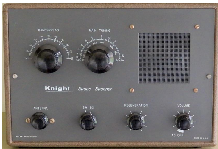
Model S-243 Allied Knight-Kit Space Spanner Short-Wave Receiver Tuned 6-17 MCS (MHz) Shortwave plus the Broadcast Band W9MXQ Collection
