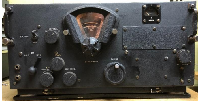
Novice Station WN9FIY, Bob Bailey, in 1970 – Now W9DYQ Military Surplus BC-348-P Receiver and Home Brew 6L6 Transmitter. The 6L6 Transmitter was a modified circuit from the 1955 ARRL Radio Amateur's Handbook. Bob refurbished the receiver and built the transmitter for his Novice station. W9DYQ Photo
