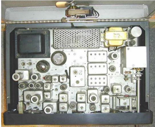
Top Inside View – HT-30 Transmitter (Front at Bottom of Picture)
