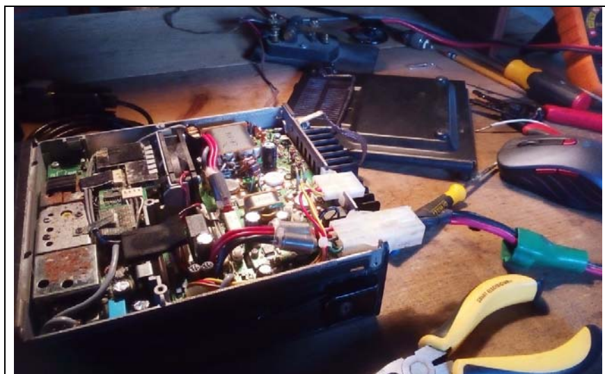
Icom 706 MKIIG with bottom cover removed
