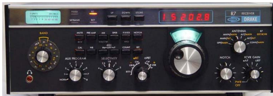
Drake R7 HF Receiver (RigReference Photo)
