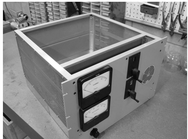
Shown is the basic amplifier panel and case prior to fabrication of the circuitry.
