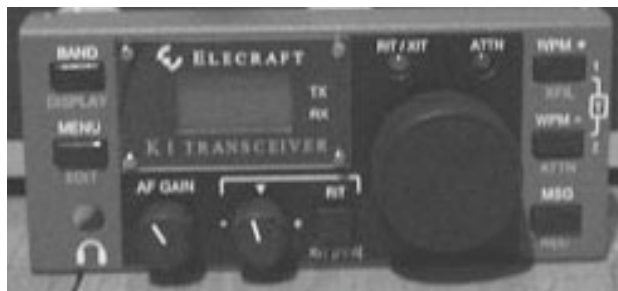
The very small dual band QRP HF Elecraft K1 Transceiver as being built by member Don Zank (AA9WP)
