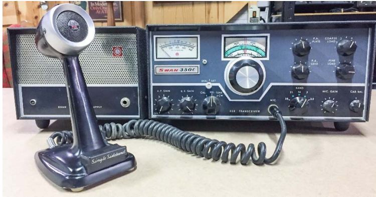
Swan 350c HF Transceiver with 117xc Speaker/PS (Shown with Turner 454C Microphone)
