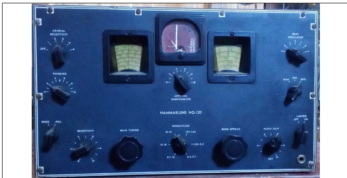
Hammarlund HQ-120X Receiver, manufactured in 1941. The front panel does not have the "X", the model number is marked on the chassis. Crystal filter controls in upper left. Calibrated band-spread dial on right. The front panel is black; the lighting makes it look blue. Photo credit: W9JI
