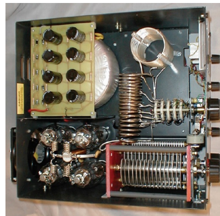
Linear Amp UK Ranger 811H Interior
