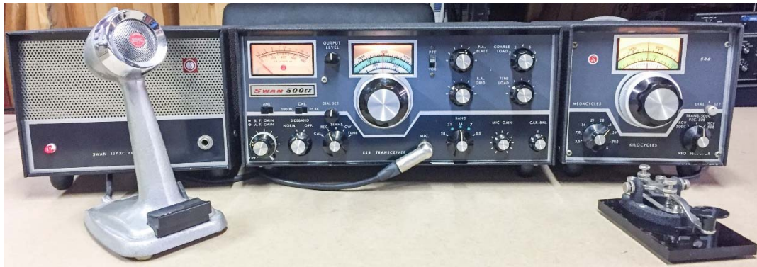
Swan 500cx HF Transceiver with 117xc Speaker/PS and 508 VFO (Shown with Turner 254C Microphone and Johnson Speed-X Key)
