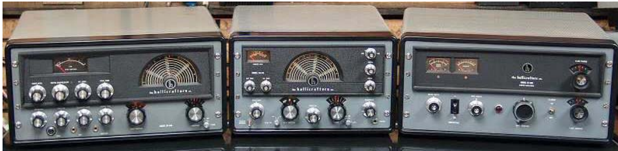
Left to Right Hallicrafters HT-32B Transmitter, SX-115 Receiver, and HT-33B Linear Amplifier
