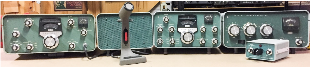
Heathkit SB-401 Transmitter and SB-303 Receiver Shown with HDP-121A 2 Microphone SB-200 Linear Amplifier, and HD-1410 Keyer (W9MXQ Shack Photo)
