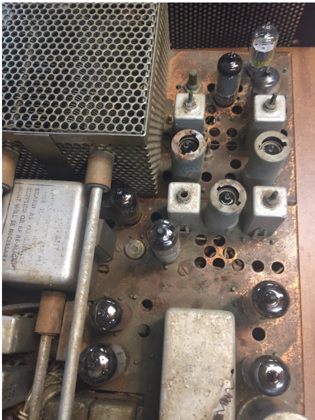
TR-4 – Copper Plated Chassis (On loan from W9JI)
