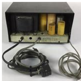
Drake RV-3 showing the AC-3 Power Supply mounted in the rear
