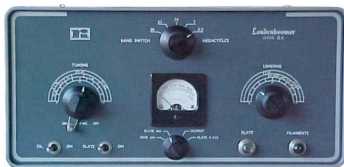
Radio Industries Loudenboomer Mark IIA 80-10 Meter Linear Amplifier (Radio Industries PS-2A High Voltage Power Supply is Separate.)
