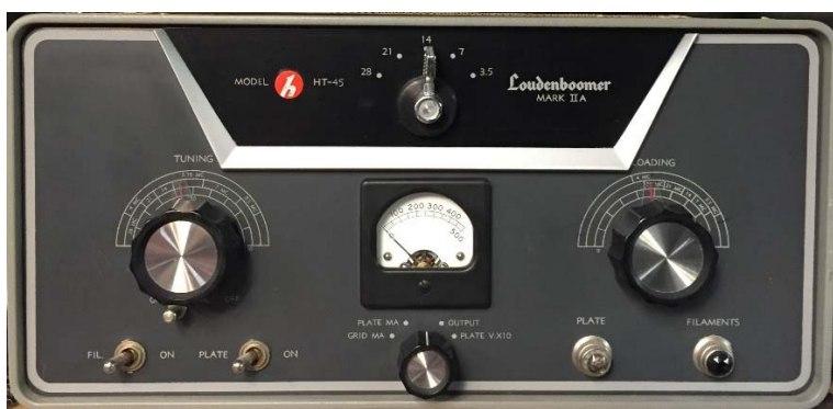
Hallicrafters HT-45 Mark IIA 80-10 Meter Linear Amplifier (Hallicrafters P-45 High Voltage Power Supply is Separate.)
