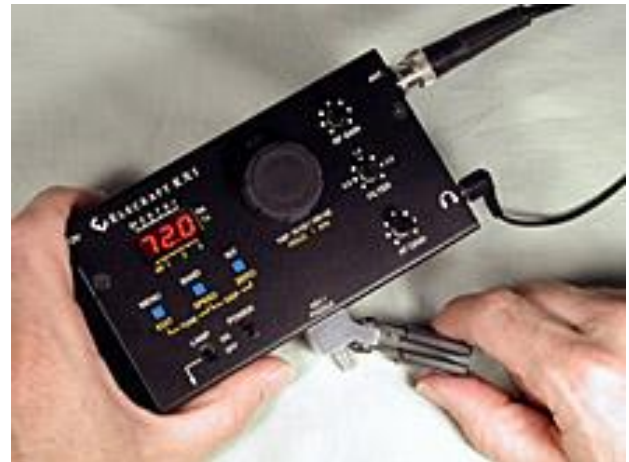
The Elecraft KX1 – a two band QRP transceiver with a keyer- receives SSB/CW & transmits CW only
