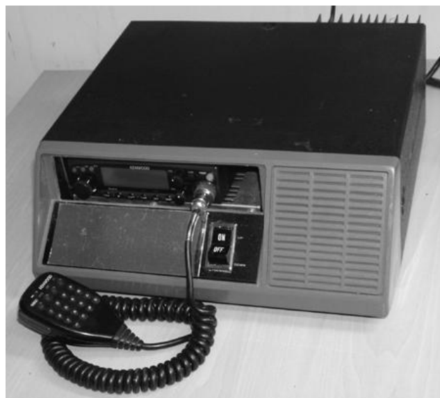
Docking station completed and with capability of accepting a variety of mobil radios.
