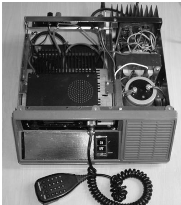
The Kenwood is installed and powered by the retained power supply and connected to the cabinets speaker
