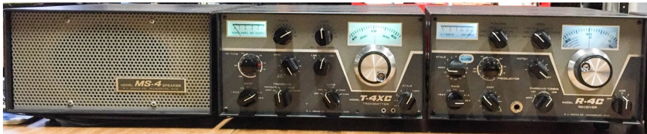
Drake T-4XC Transmitter and R-4C Receiver with Drake MS-4 Speaker Console
