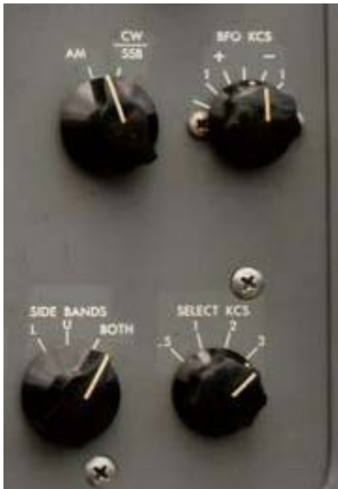
HQ-170 (HQ-180 was similar) SSB and CW were the same mode switch position (see upper left) WØUI
