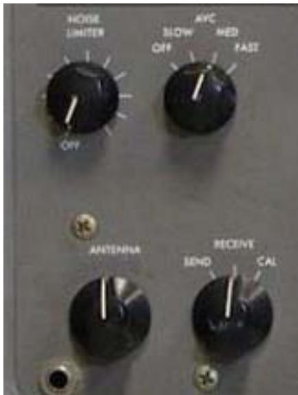
HQ-170 or HQ-180 Receiver Lower left corner of Front Panel This radio has no NS-1 Noise Silencer, only the standard NOISE LIMITER W9MXQ
