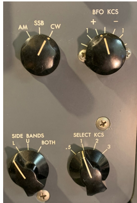
HQ-170A (HQ-180A was similar) SSB and CW were separate mode switch positions (see upper left) W9MXQ
