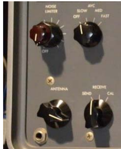
HQ-170 or HQ-180 Receiver Lower left corner of Front Panel See Maroon concentric NS-1 Level Knob on the NOISE LIMITER knob. W9MXQ
