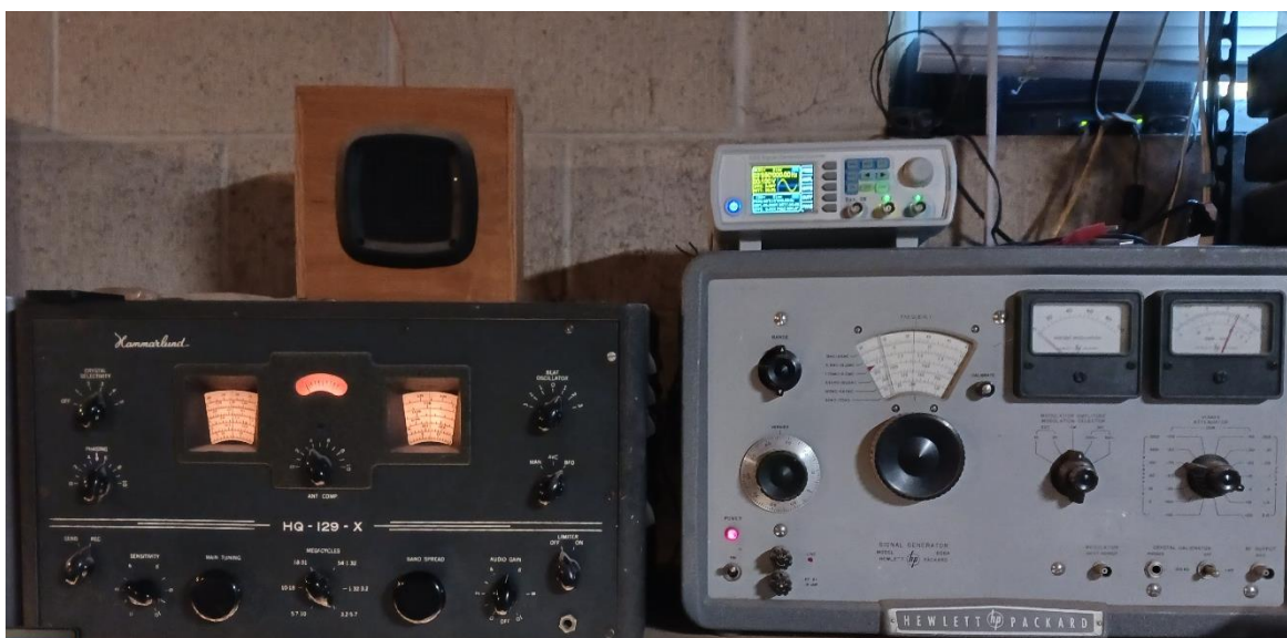
The signal generator and radio can be connected to the antenna bus located overhead. (Hammarlund HQ-129, HP Model 606A Signal Generator, and Koolertron Signal Generator)
