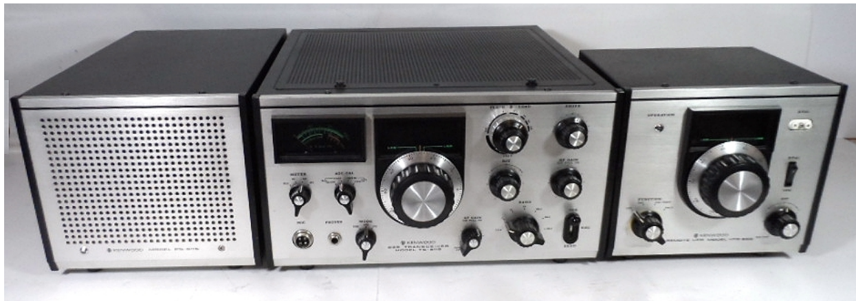
Kenwood TS-511S HF (80-10 Meter) SSB/CW Station TS-511S HF Transceiver (Center) with PS-511S AC Power Supply/Speaker (Left) and VFO-5SS External VFO (Right)
