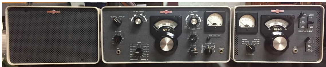
Collins KWM-2 Transceiver (Center), 312B-5 Remote VFO (Right), and 516F-2 AC Power Supply (Left)
