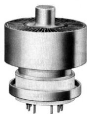
RCA (now Burle) 8122 Ceramic Tetrode 400 watts Plate Dissipation (OEM in the National NCL-2000) W9MXQ
