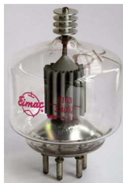
Eimac 3-400z Glass Triode 400 watts Plate Dissipation (OEM in the Drake L-4 and in the Hallicrafters HT-45) W9MXQ
