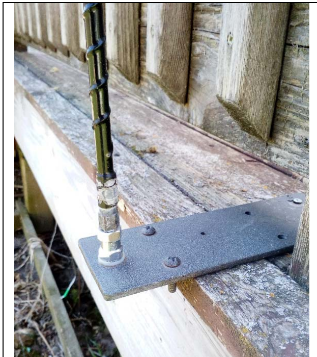
Mounting bracket for Hamstick antenna (photo by W9JI)
