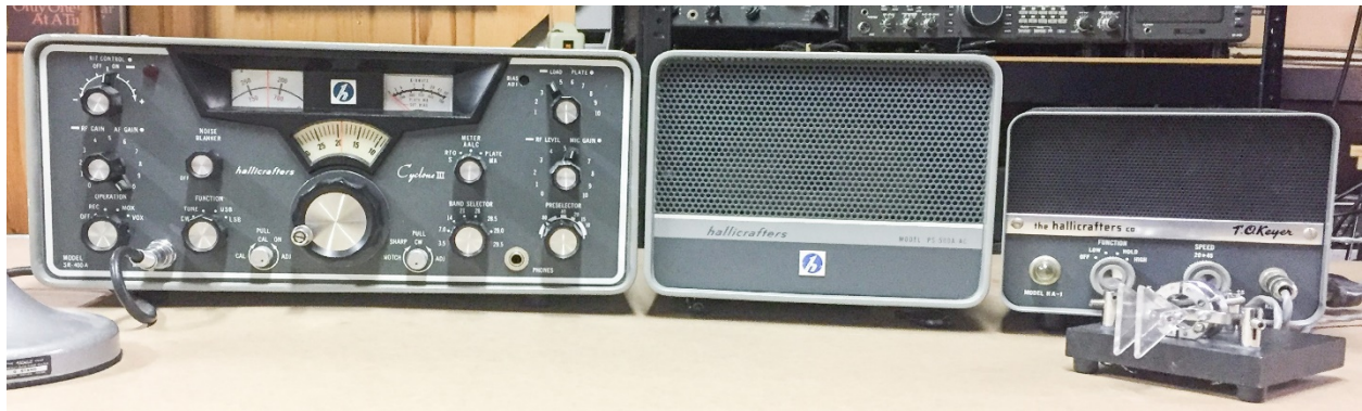
Hallicrafters SR-400A Cyclone III HF Transceiver Shown with PS-500A-AC AC Power Supply/Speaker and HA-1 Electronic Keyer W9MXQ Shack Photo
