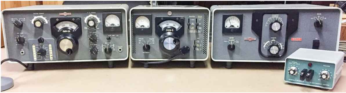
Collins KWM-2A HF Transceiver in the Original Article With Collins 312B-5 and 30L-1 Linear Amplifier – and Heathkit HA-1410 Keyer W9MXQ Shack Photo
