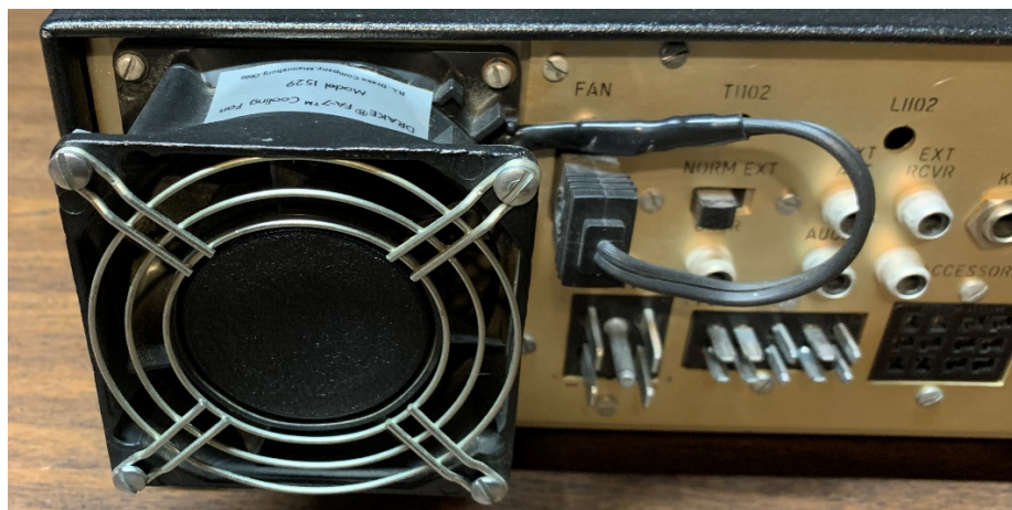
Drake FA7 Fan installed on a TR7 Transceiver Note Drake installed power-lead to molded non-polarized plug on cord.
