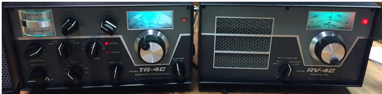
Drake TR-4C 80-10 Meter SSB/AM/CW Transceiver and RV-4C External VFO (Part of the Drake Collection at W9MXQ)
