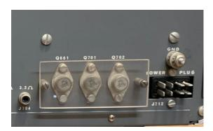
This view shows the lower right-hand corner of the HQ-215 Rear Panel. Note the Cinch-Jones Power Plug, the Ground Lug, the External Speaker Connector, and the three sheet Plexiglas™ isolated power transistors. Transistor Q601 is the radio's Power Supply Pass Transistor. All three transistors are RCA 40310 devices.
