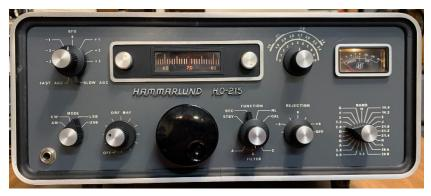
The front panel is conveniently laid out and is somewhat reminiscent of the Collins 75S-3C on which its design is based. Reviewing the important controls, one can see the prominent main tuning knob. It is nice to see that this radio uses generally available open stock
