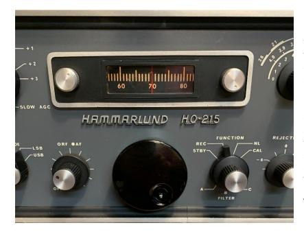
Here is a center front panel view of the HQ-215. Note the visible edge of the dial drum through the opening above the main tuning knob. This frequency line markers are 1 kHz apart for good detail in reading an analog dial. The knob to the left of the window is to adjust the dial pointer for exact frequency readout. The knob to the right adjusts lamp brightness.
