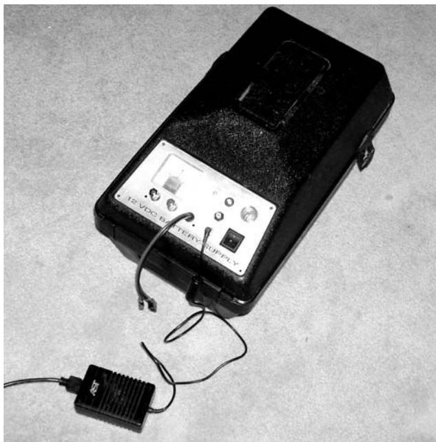
The 14 VDC laptop computer power supply used as a charger had the output cord adapted to Anderson “power-pole” connectors to facilitate charging. There is also an adapter for the “cigar lighter” type receptacle to all use with “power- poles” and other types of power connectors.
