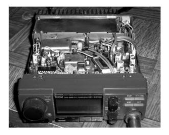
Back at the bench, armed with new information, I pulled the circuit board out of the radio. The oscillator circuit has a cover over it. I thought about what the tech said about needing to heat the case, as I desoldered the tabs. A medium screwdriver finally popped the cover off, to reveal a blank circuit board! The oscillator was inside the cover, well soldered in, and I had broken off four leads with my screwdriver in removing it!
